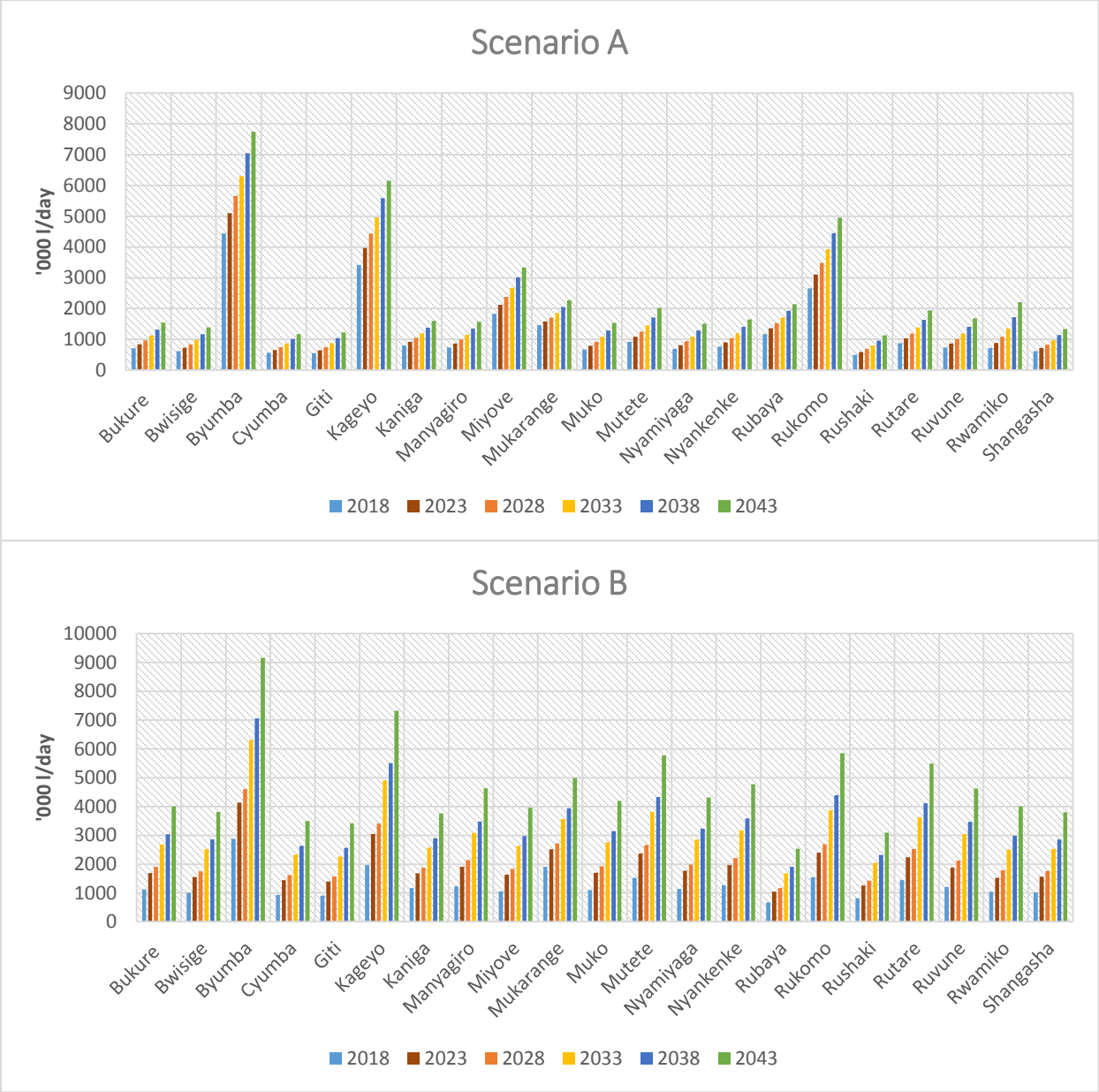
Figure 29: Water demand for Gicumbi District per sector estimation (A) conservation water consumption rate scenario; (B) scenario based on National Water Master Plan consumption rate
